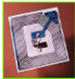
Figure 10: An identification transponder integrated on an anti-theft sticker.
