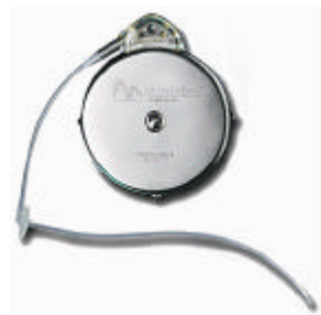
Figure 7: Implantable Insulin Pump
